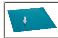
step 1: glue the dolly on the paint coating
