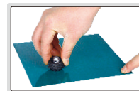
step 2: cut the paint around dolly by using ring cutter
