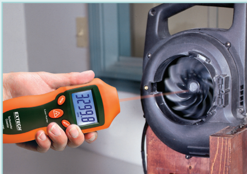
Non-contact fan blade RPM or REV testing
