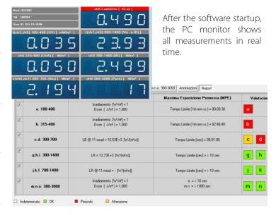
Through the **DeltaLog13** software downloadable from the Delta OHM website, you can **configure** your HD2402 (calendar, date, time, start time and logging time), **set** that the proper measurement ranges and **perform** your measurement campaign.
