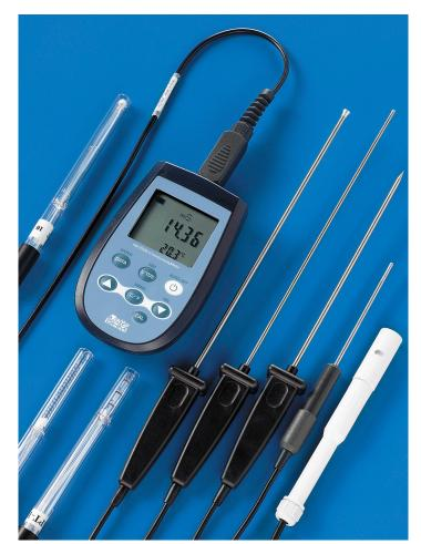
HD2306.0 CONDUCTIVITY METER - THERMOMETER
