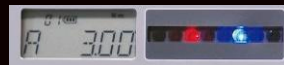
Preset Tightening Mode (Red LED shows the level of the applied torque)
