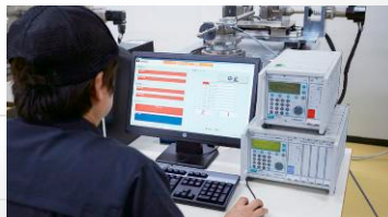
Calibration of 100N·m Torque Wrench Calibration Machine by 100N·m Designated Secondary Standard Equipment
