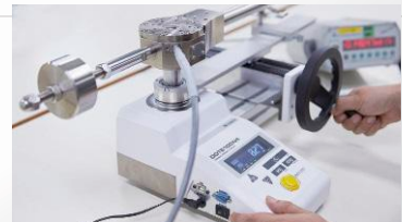
JCSS calibration for digital torque wrench tester by maximum 100N · m reference torque wrench
