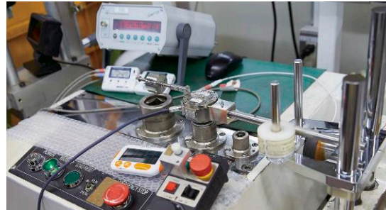
Calibration of tester by a reference standard in inspection room.
