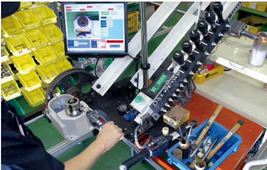
Tightening Assurance System at Omori factory
